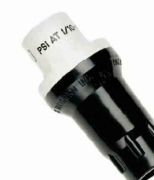
Pressure Reducer Pressure reduced to 30 psi for proper operation of drip system. Install downstream of valve.
