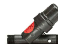
In-Line Filter for Dripline Internal screen/ mesh prevents clogging of drip components. Install downstream of valve.
