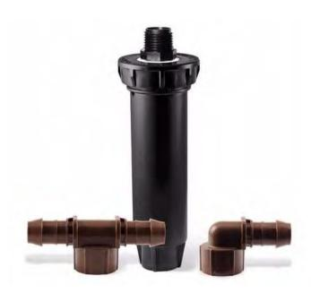
Rain Bird® 1800-RETRO is the easiest and fastest way to convert a conventional spray zone to a low-volume irrigation zone. The 1800 Retro internal assembly is easily installed into any existing 1804, 1806, or 1812 spray head bodies to retrofit existing system to Xerigation products.
