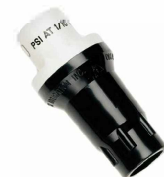
Pressure Reducer. Pressure reduced to 30 psi for proper operation of drip system. Install downstream of valve.
