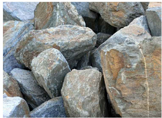
RED MOUNTAIN BOULDERS: Landscape boulders ranging in size 9", 12", 18" to be used throughout.
