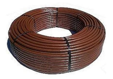
Netafim continues to be the leader in innovation in the Landscape & Turf dripline market by introducing Techline CV manufactured with post-consumer recycled polyethylene. Techline CV Dripline has the most technologically advanced embedded/inline emitter/ dripper available. Techline CV's Check Valve feature keeps water from draining out of the dripline after zone shut-down.
