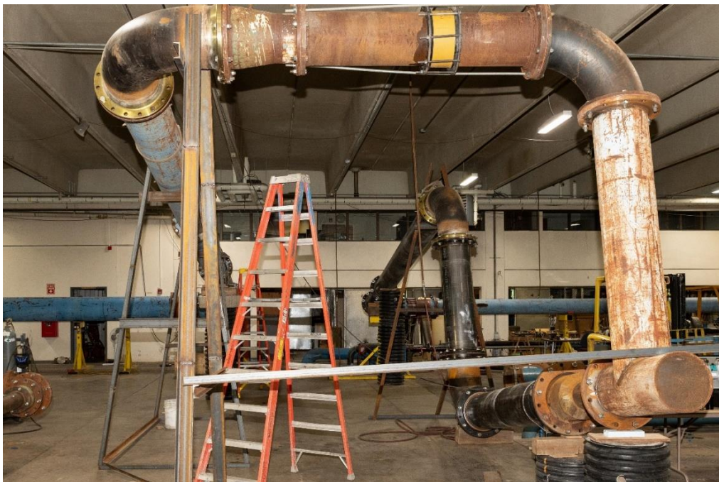
Figure 1 Physical Hydraulic Model of OC-70
