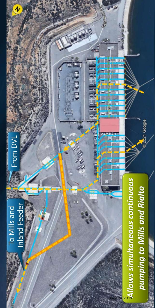
Tunnel Portal Arrowhead Proposed El. 1875' Intertie Inland Feeder / Rialto Pipeline Intertie Proposed ~El. 1830 Intertie and easier operation Allows higher flow DWR's Devil Canyon Second Aferbay El. 1930
