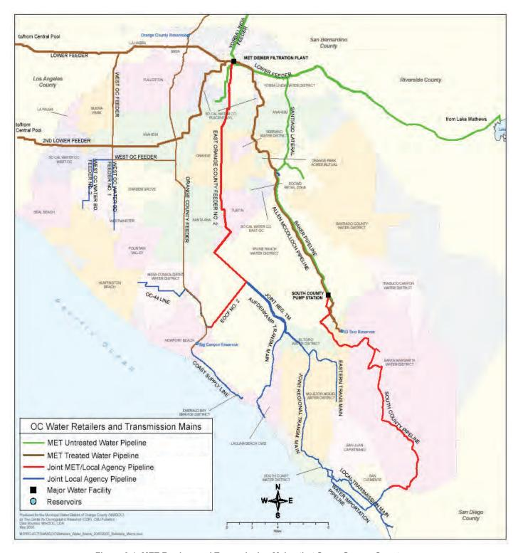
Figure 6-4: MET Feeders and Transmission Mains that Serve Orange County
