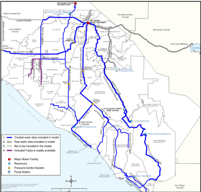
Linear water system infrastructure to be included in the model build of the MWDOC system as determined by Black & Veatch and MWDOC during Phase 1.
