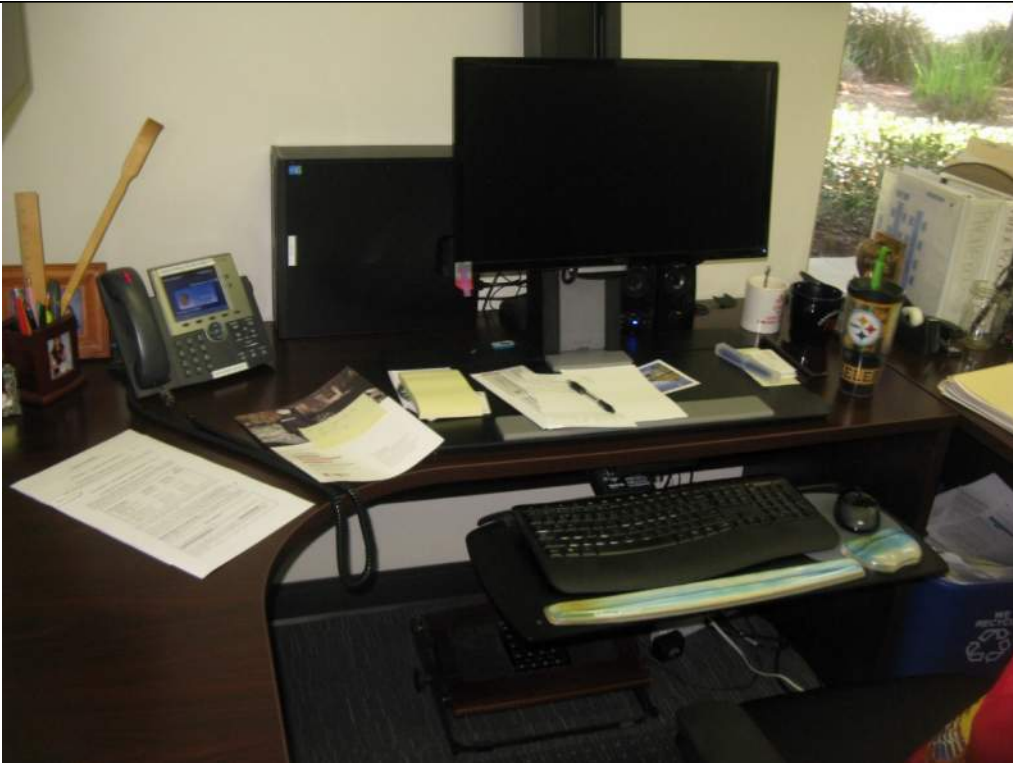
Photo 19: Typical Unanchored Office Computer Equipment
