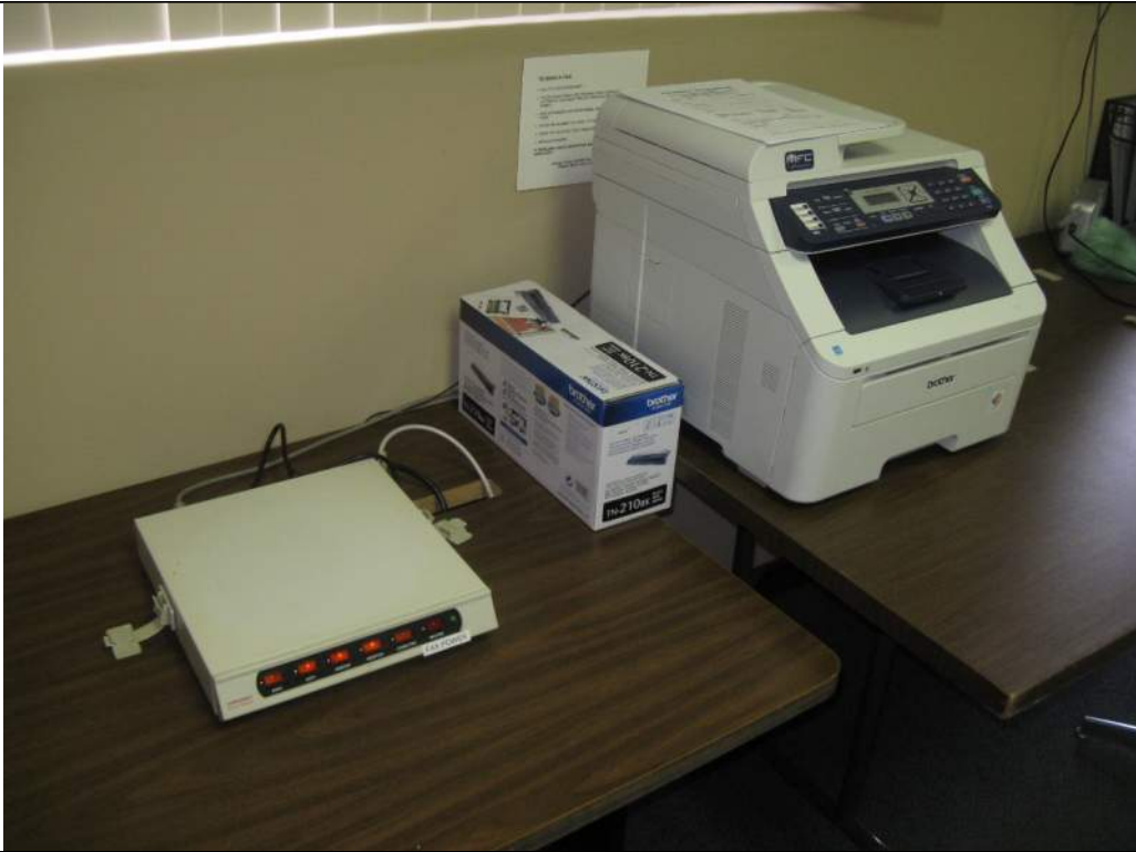
Photo 33: Unanchored Computer Equipment
