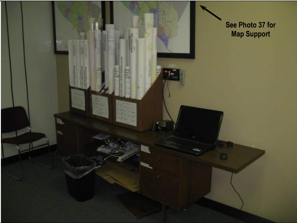
Photo 34: Unanchored Computer Equipment & Documents
