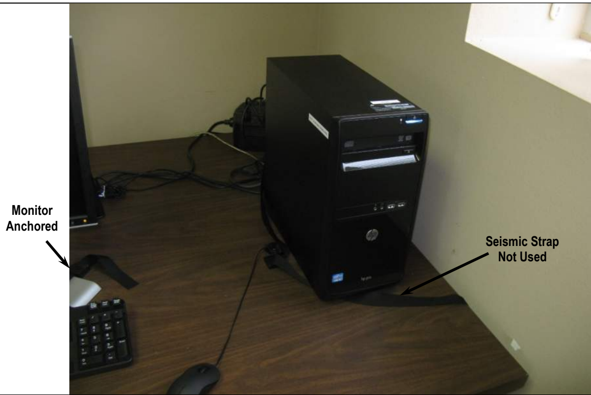
Photo 32: Unanchored Computer Equipment
