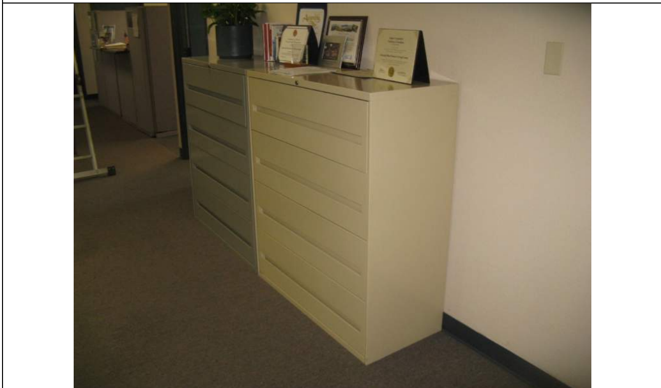
Photo 22: Unanchored Tall Narrow Contents in Hallway
