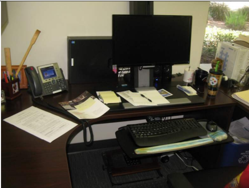
Photo 19: Typical Unanchored Office Computer Equipment
