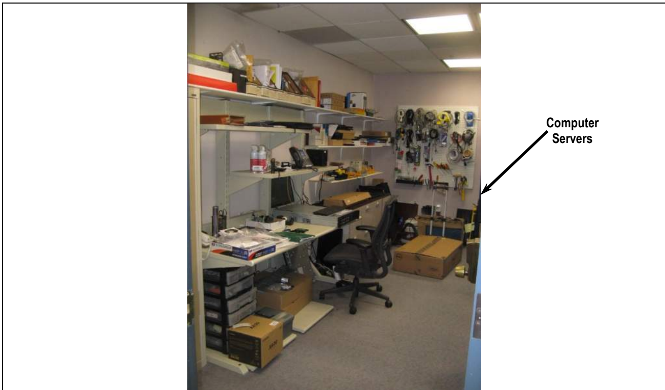
Photo 21: Unrestrained Contents in Computer Server Room
