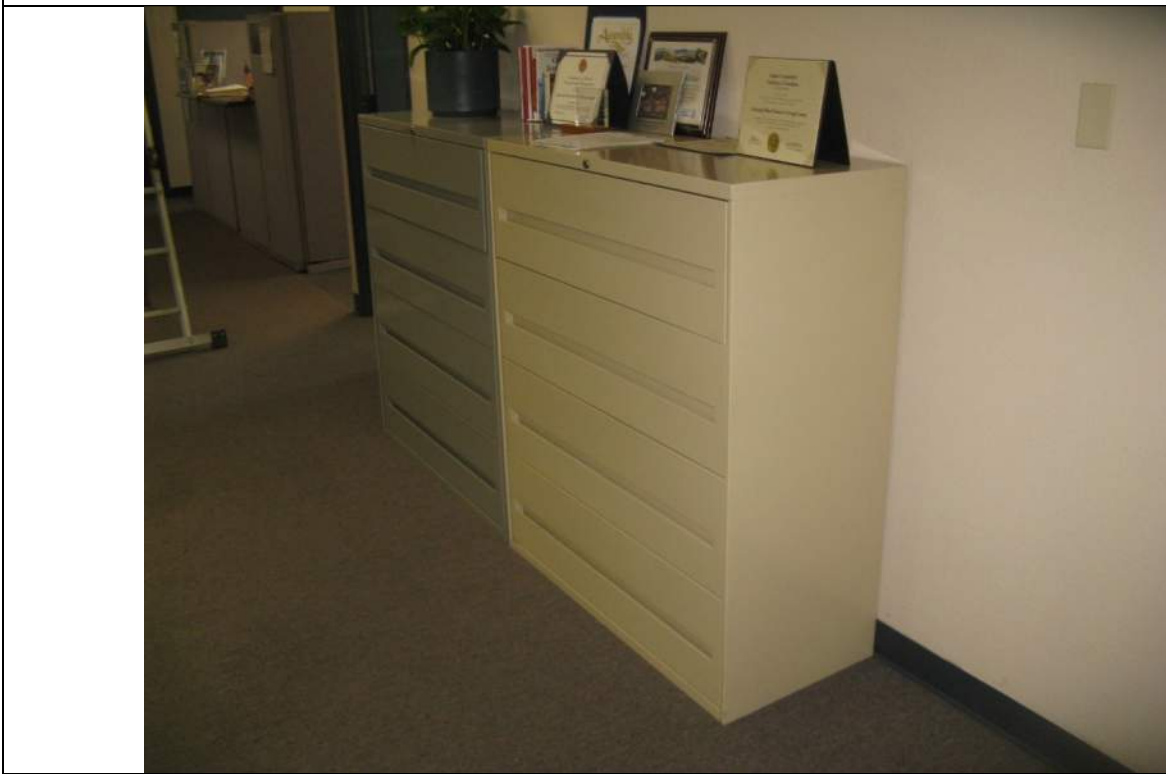
Photo 22: Unanchored Tall Narrow Contents in Hallway
