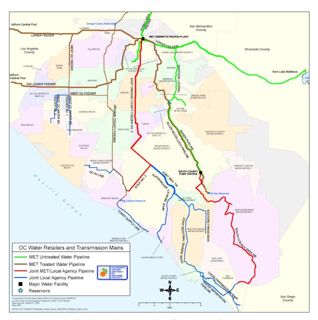
Figure 3-4: Metropolitan Feeders and Transmission Mains Serving Orange County
