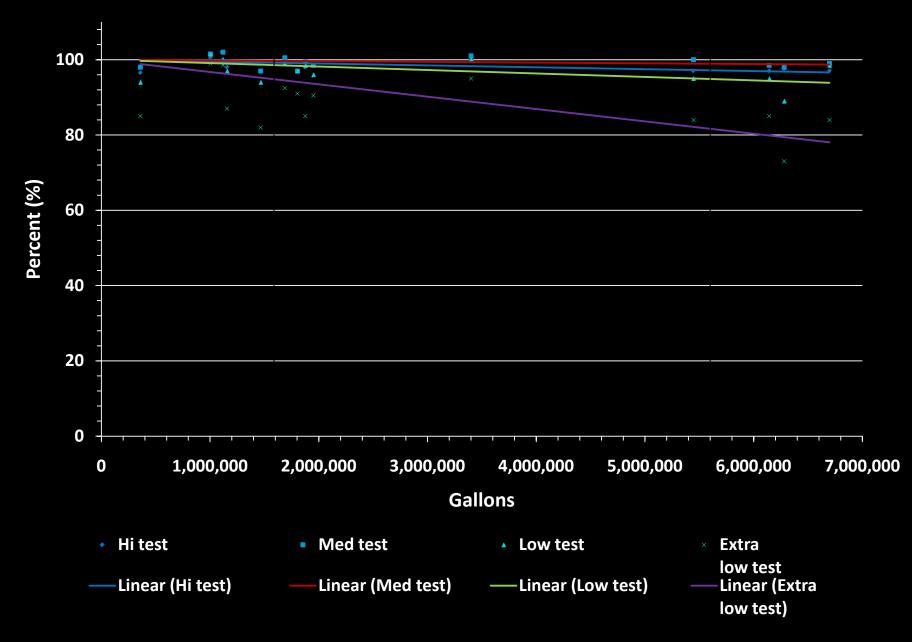
Figure 4.4: 1 1/2-Inch Meters Cumulative Flow vs. Accuracy
