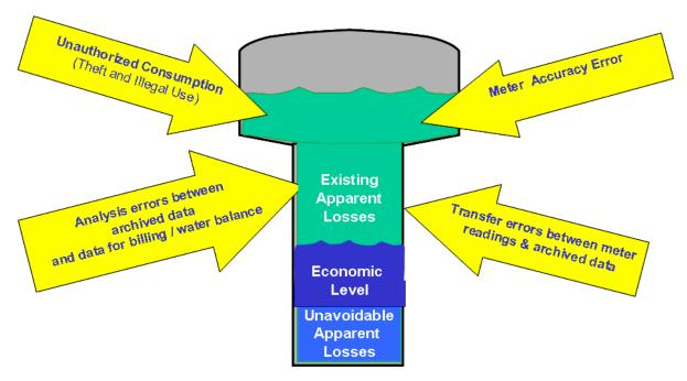
Figure 2-3: The four basic methods of managing Apparent Losses
