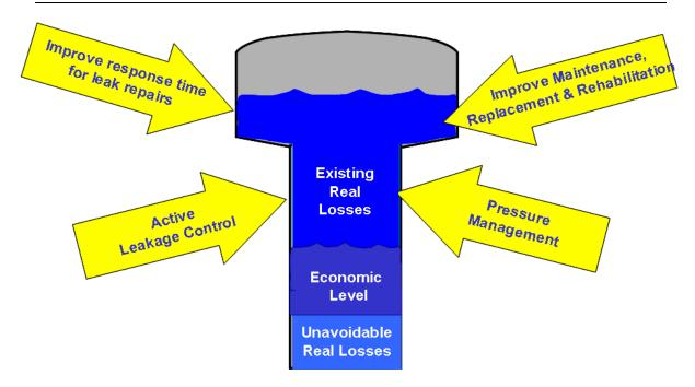
Figure 2-2: the four basic methods of managing Real Losses
