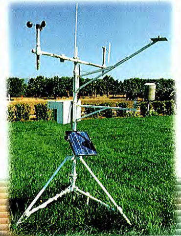
California Irrigation Management Information System (CIMIS) weather station measuring daily ET o .
