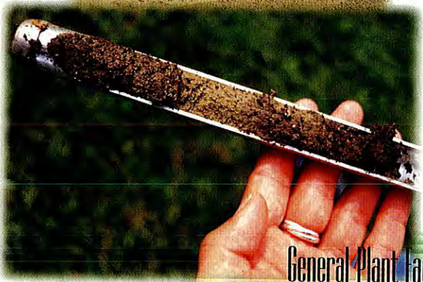
Soil probes help water managers assess irrigation schedule impacts in the soil.
