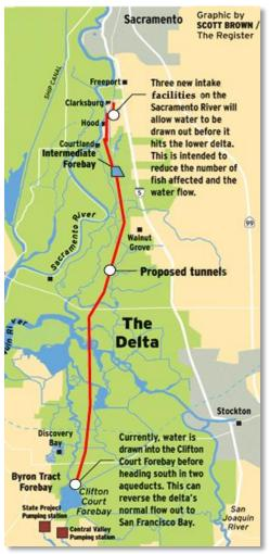
Current pumps are powerful and cause reverse flows which trap endangered fish and pull them towards predators. State of the art construction techniques, advanced fish screens, and tunneling improvements, promise minimal impact on Delta species.
